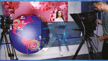
RECKEEN 3DSPRO X8 has an ability to receive signals from up to four cameras, via SDI or HDMI, each in 4kp30 resolution. Their signals are keyed independently in high quality, thanks to four high-end chroma keyers. NDI inputs are also available to enable a more remote workflow.
